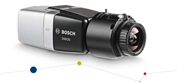
The DINION IP starlight 8000 MP captures images at 5 megapixel resolution even under extreme low-light conditions, giving amazing images in fine detail. With a remarkably high frame rate of 30 frames per second, you can capture fast moving objects in high resolutions regardless of the lighting conditions or time of day. The camera produces multi-megapixel full-color video in near darkness, and delivers detailed monochrome images where other cameras show no image at all.
