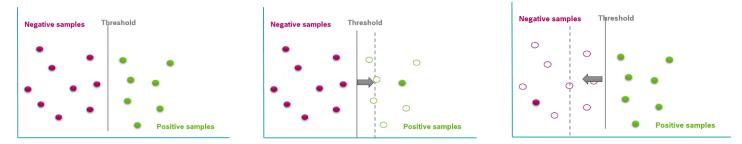
Thus, only by giving enough positive and negative samples will the threshold be set correctly. Note that in real examples it is often not possible to find such a perfect separation and some missed detections as well as false detections will occur, especially if something has not been seen before in the training.
