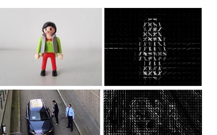
Only objects with distinct edges can be detected, and the edge pattern needs to be sufficiently different from the background as well as all other objects in the field of view. Small details are easily lost. Thus, a person wearing a helmet or safety vest cannot be distinguished from one without. Similarly, a sports car would not be differentiable from a SUV.
